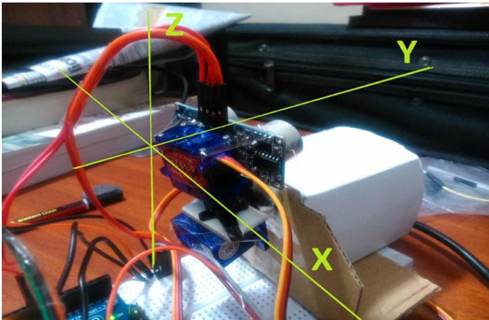
The rotation of the second servo (the servo on top) gives the value of the angle  $\alpha$ . The angle of rotation of the base is  $\beta$ .
