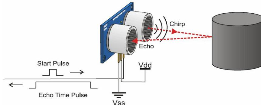
We control the ultrasonic wave generation by sending a pulse to the pin connected to the "Trigger" pin of the sensor board. On receiving the echo, the sensor sends an echo time pulse to the arduino (through the "Echo" terminal of the sensor board). The length of this pulse is proportional to the distance to the surface.
